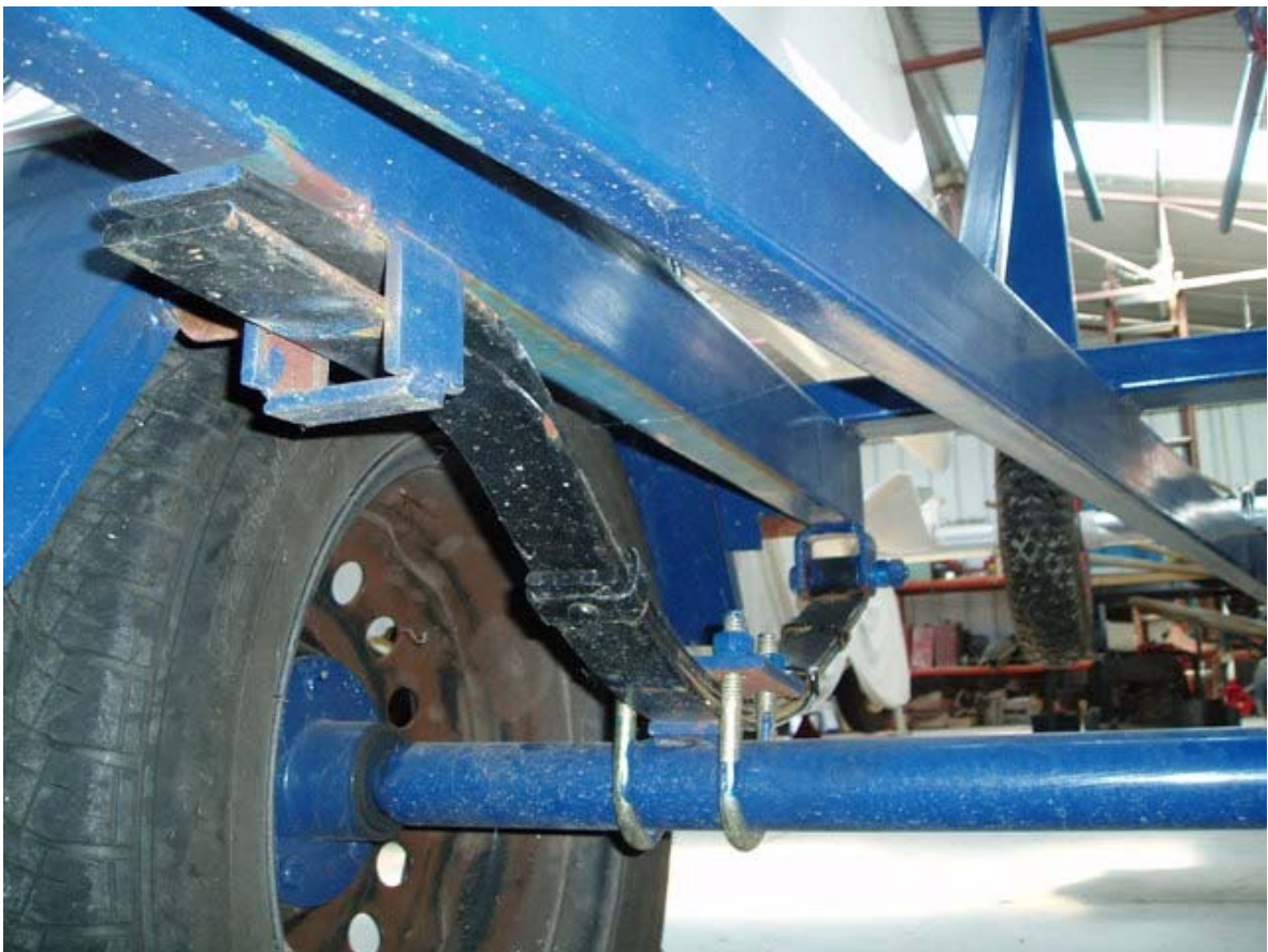
Underside view of axle support
