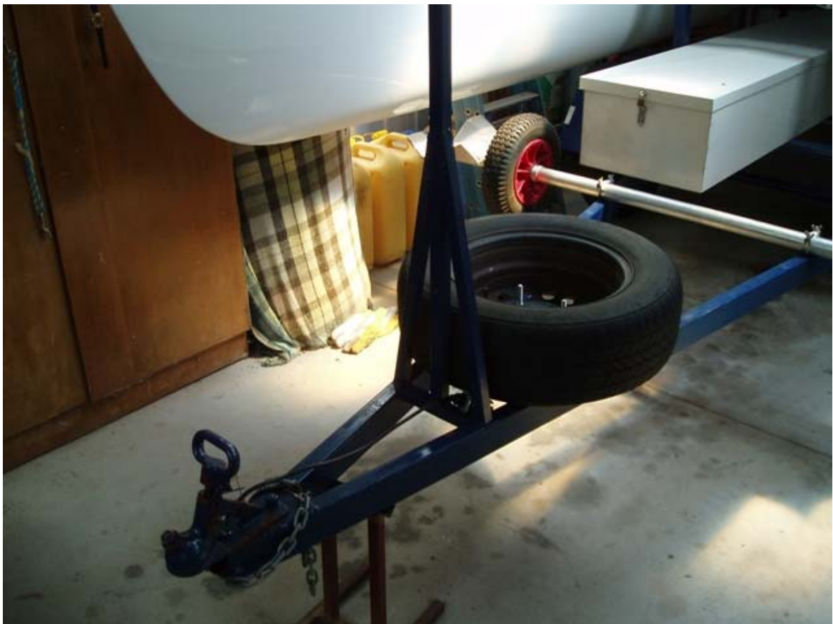
Draw bar, mast support, spare wheel and beach trolley
