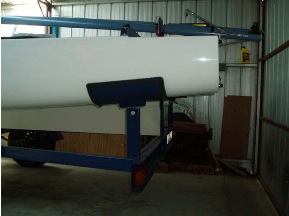
Rear hull support from the outside
