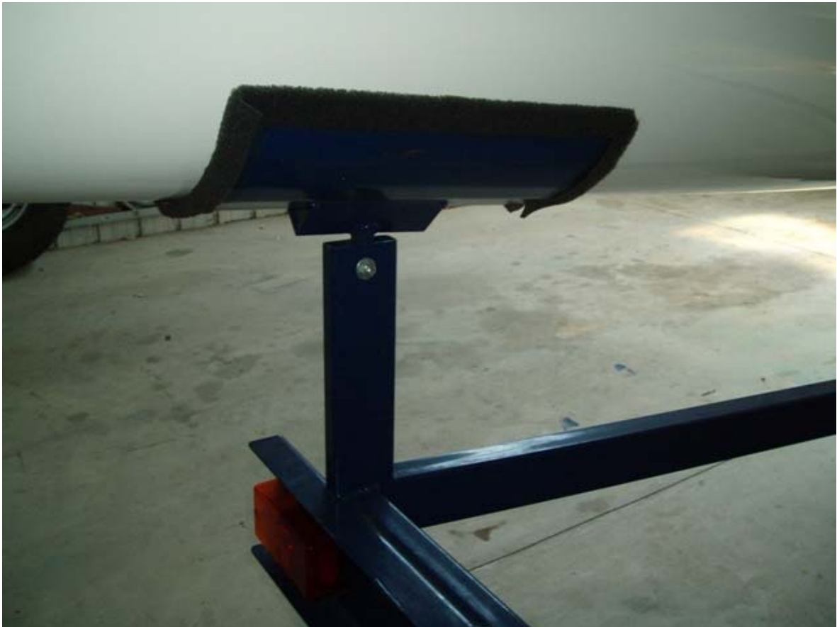
Rear hull support from the inside
