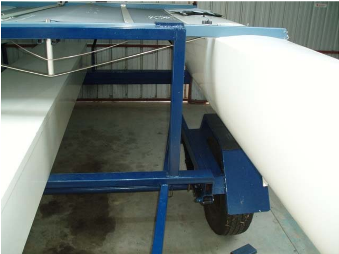
Front view of main beam support and axle attachment
